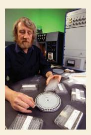
Soil samples collected from the field are loaded into a carbon/nitrogen analyzermass spectrometer carousel to measure how much carbon plants have pulled from atmospheric carbon dioxide and stored in soil organic matter.
